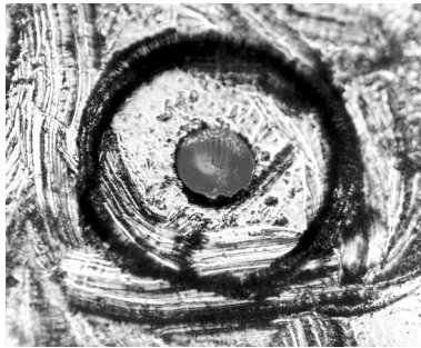
Figure 7-7. Damage from improper cleaning.
